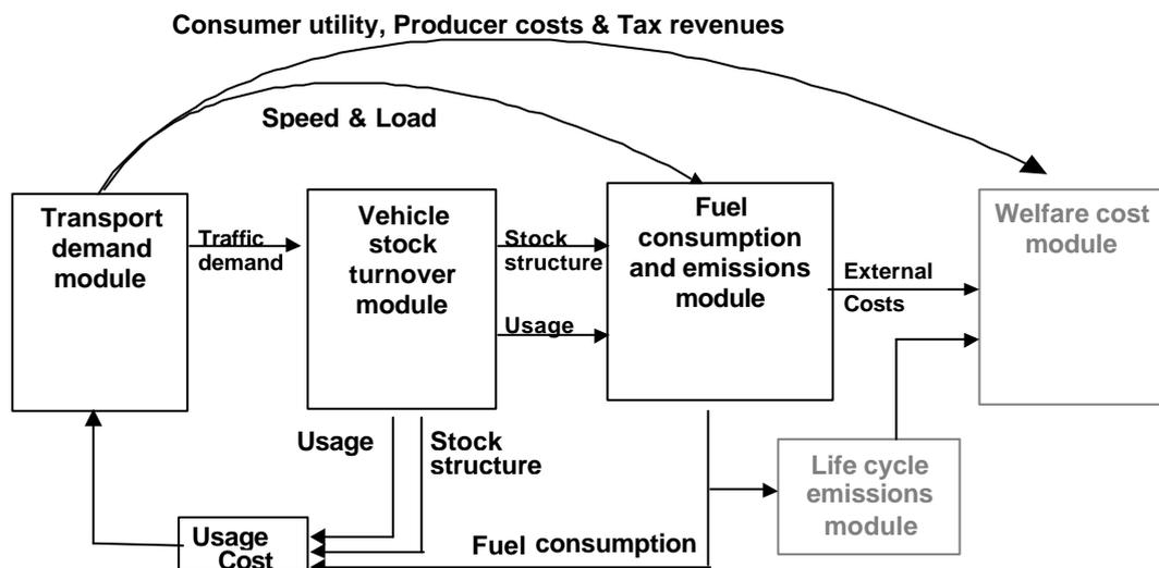
Figure 1 : Modular structure of TREMOVE 2 Model.
