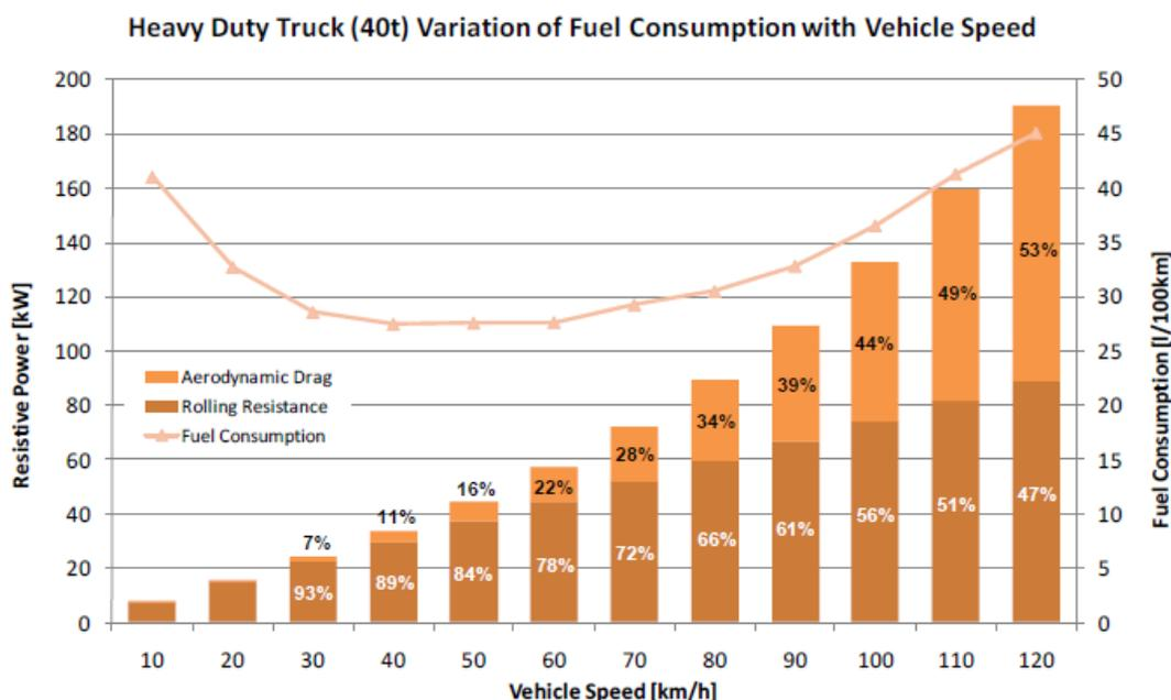
Figure 6: Fuel consumption as a function of vehicle speed
