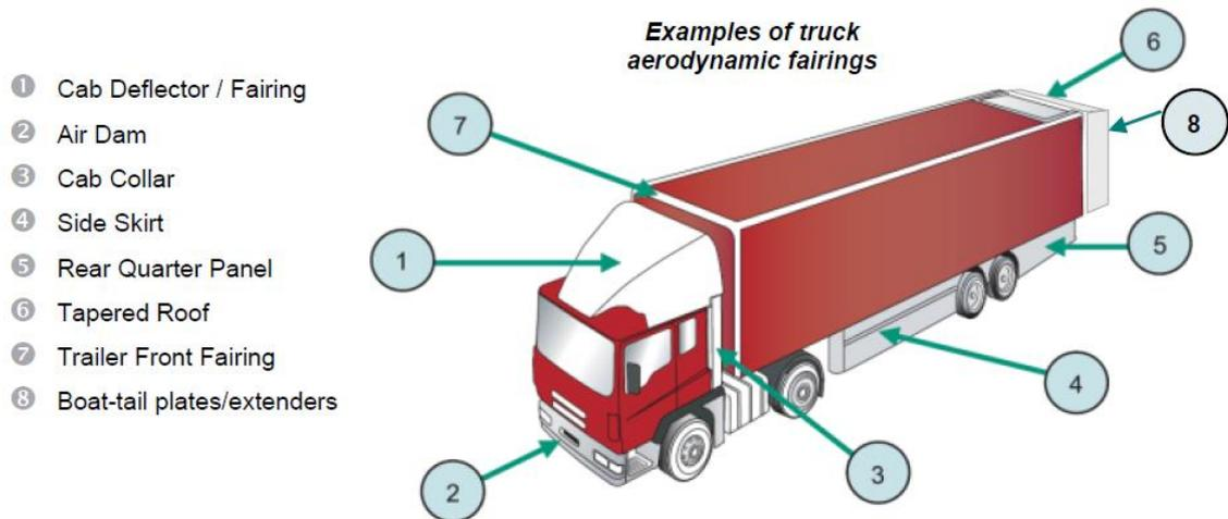
The improvement in aerodynamic properties should reduce fuel consumption of new vehicles by 4% (long haul) or 3% (regional delivery), half of which can be realised by OEMs; the other half is to come from trailer/body builders.
