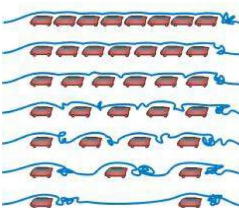
Figure 8: schematic view of the concept of vehicle platooning
