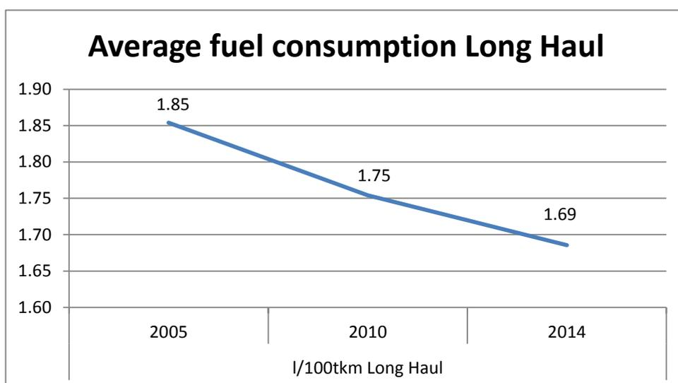
Figure 3: Fuel consumption of Long Haul reference vehicles
